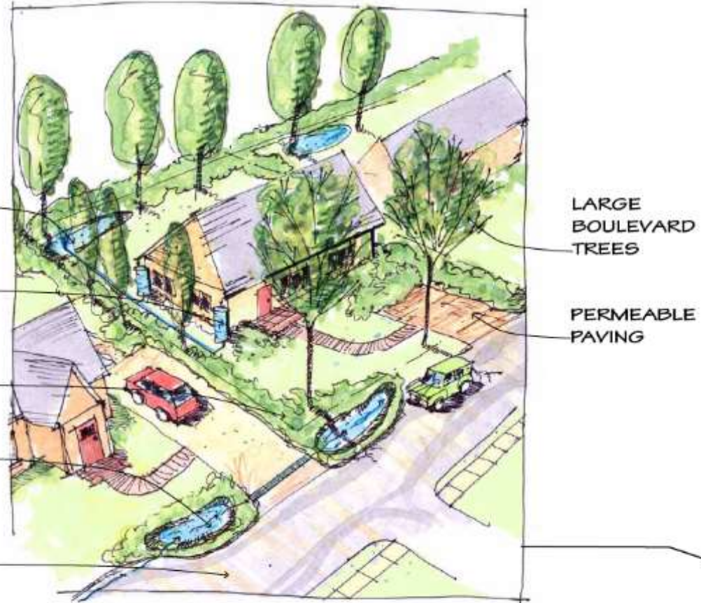
RESIDENTIAL LOW-IMPACT RETROFIT
